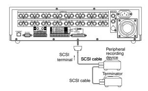
When connecting a peripheral recording device, the SCSI TERMINATION switch must be set to OFF.
